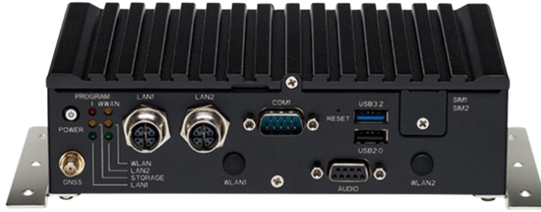
Figure 5.4: The nROK 1030 onboard edge device used to execute MobilityNebula queries on trains
