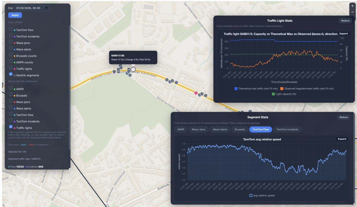
Figure 7.6: Avenue Charles-Quint segment with the traffic-light layer enabled. The Traffic Light Stats panel on the right plots capacity for the selected signal group SAB01/3 against theoretical maximum traffic and against observed magnetometer traffic. The Segment Stats panel below carries the TomTom relative-speed curve for the same corridor in the same window.
