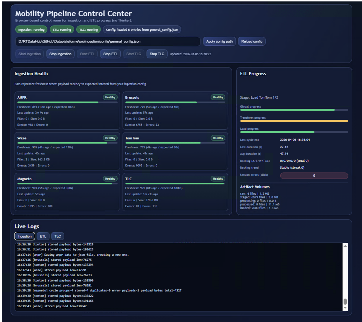
Figure 7.1: The Mobility Pipeline Control Center on the deployment server. The page consolidates configuration, start/stop controls, per-source ingestion health, ETL progress, and live logs into one browser view.
