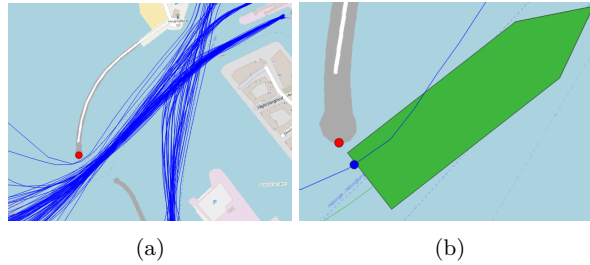
Fig. 5.18: (a) Entrance to the port of Helsingborg, with the query point in red and the vessel trajectories in blue. (b) Visualization of the vessel with the closest approach in both the point (blue) and polygon (green) representation.
