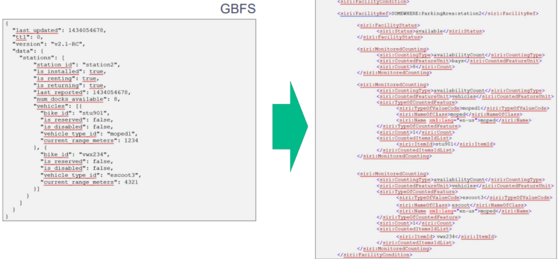
Figure 4.6: Mapping GBFS to NeTeX/SIRI 14
